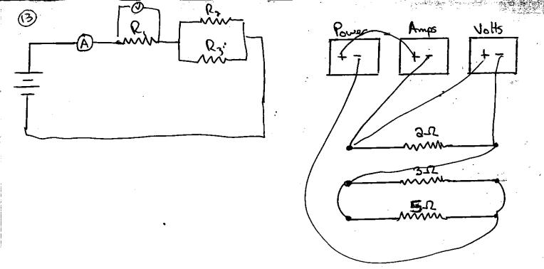
Resistor R<sub>1</sub> is connected in series with the parallel combination of R<sub>2</sub> and R<sub>3</sub>. The ampmeter measures current out of the power supply and a voltmeter is reading the voltage across R<sub>1</sub>. Complete the schematic diagram and complete the chart below according to the circuit.
