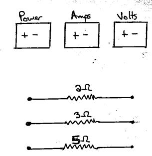
Resistor  $R_1$  is connected in series with the parallel combination of  $R_2$  and  $R_3$ . The ampmeter measures current out of the power supply and a voltmeter is reading the voltage across  $R_1$ . Complete the schematic diagram and complete the chart below according to the circuit.
