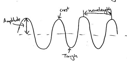
wavelength (1) - the distance between 2 successive crests or troughs. Measured in meters
